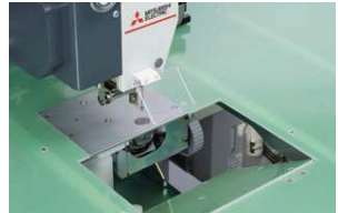
The bobbin can be replaced from the top
