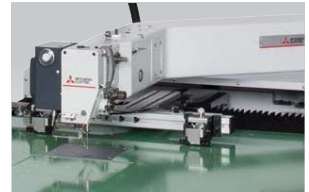
Easy maintenance! New arm-shaped, glass epoxy slide plate
